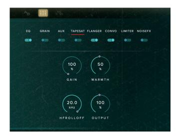
Tape Saturation emulates gentle compression and distortion of recording to tape.
