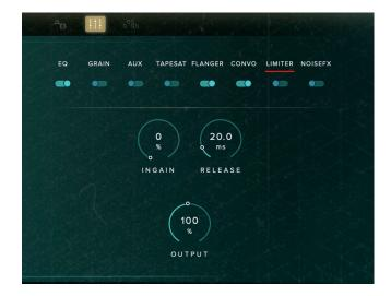
Limiters are a safeguard against clipping of the overall output signal, with a ratio of 1.100 and a fast attack.
