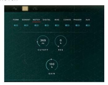
Similar to Peak however the Notch Filter cuts two bands either side of the cut off point.
