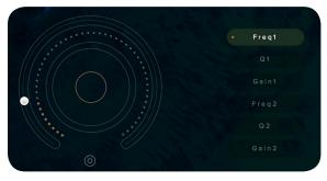
Tip: Right click on any of these controls to assign them to a MIDI controller. Remember that if you assign a MIDI controller to a parameter via the knob, the MIDI controller will follow the parameter rather than being permanently assigned to the knob.
